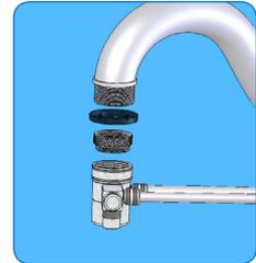
Diverter Valve Attachment with adapter
